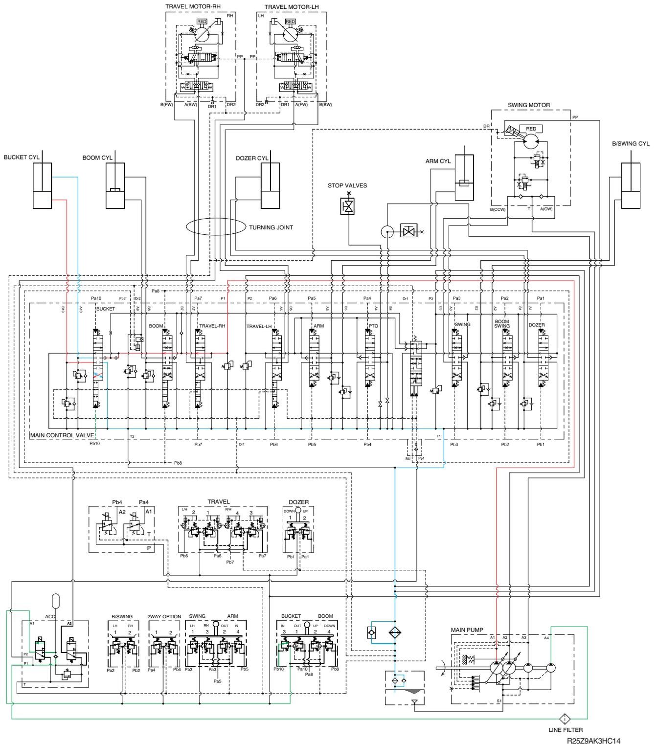
When the right control lever is pulled left, the bucket spool in the main control valve is moved to the roll in position by the pilot oil pressure from the remote control valve.
